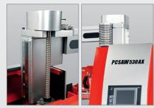
Servo-electric ball screw drive
