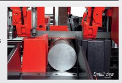
The use of a SMARTCUT 41 mm band saw blade with only 0.9 mm blade thickness specially developed for this machine type, reduces the waste by 25 %, which is particularly advantageous with respect to the efficiency during sawing of expensive materials. This makes the robust, columnguided AMADA PCSAW 330 particularly interesting for large series.
