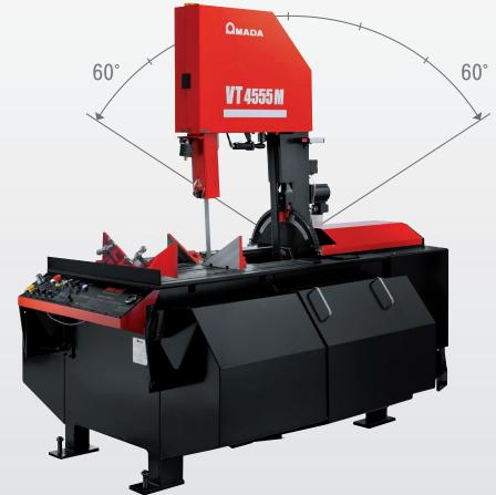
A truly universal machine capable of making virtually any conceivable straight or miter cut (60° left and right VT 4555 M / 45° left and right VT 4555). Available in both standard and high column models with or without the optional 3° column (VT 4555). VT 4555 M has adjustable cant as standard (90° or 3°). VT 4555 M has electric power tilt, VT 4555 has mechanical power tilt.
